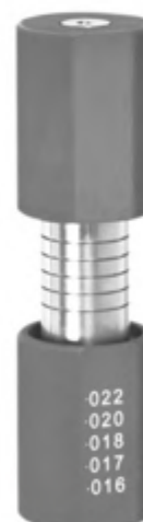
215-0072 Arch Turret with 5 wire-slots .016", .017", .018", .020" and .022"
